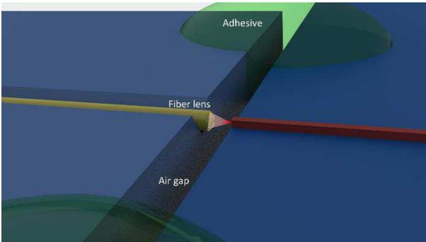
Figure 3. Close view of fiber lens coupling.
