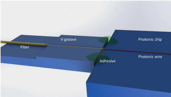
Figure 1. Typical configuration of fiber-to-chip coupling using fiber lens. The tip of the fiber has to be kept clean from the glue.
