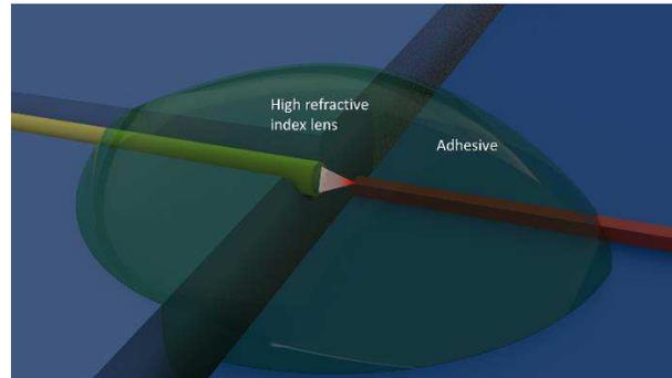
Figure 4. Close view of immersion coupling with high refractive index fiber lens.
