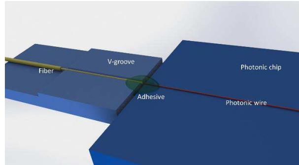
Figure 2. Fiber-to-chip coupling using high refractive index lens. Adhesive covers the point of coupling and acts as immersion.
