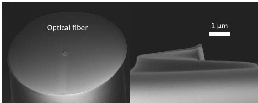
Figure 1. SEM images of the vortex phase plate on a fiber.
